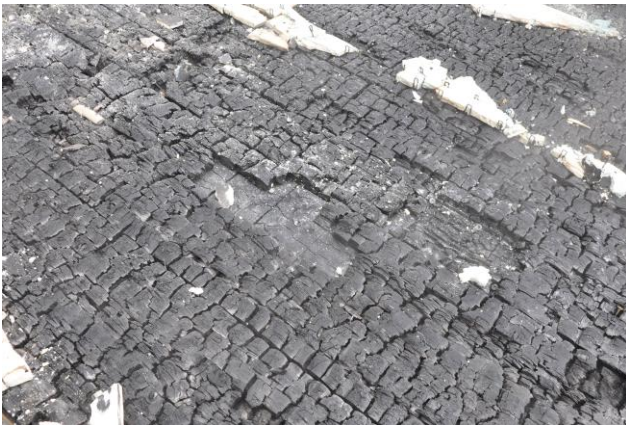
Fig. 2: char layer of an 80 mm CLT element, originally clad with fire protection plasterboard, after a large-scale fire test
