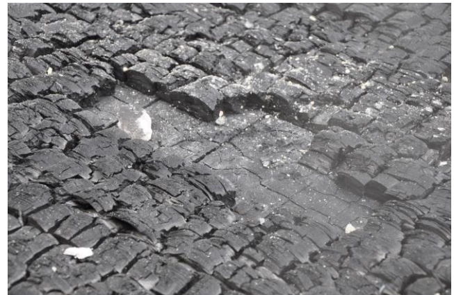
Fig. 2: char layer of an 80 mm CLT element, originally clad with fire protection plasterboard, after a large-scale fire test
