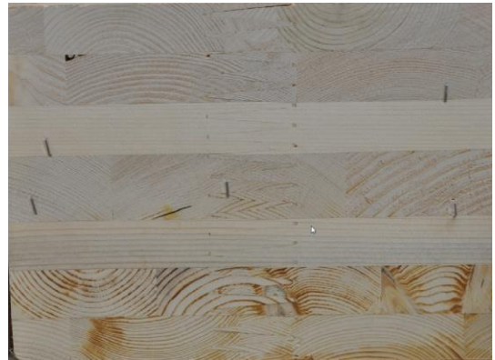
General finger joint = finger joint over the entire thickness of a panel
